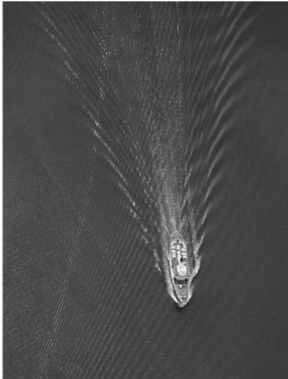
FIGURE 14.35 (a) A shock wave trails from a supersonic aircraft. The plane is flying low over the ocean, and the humid air condenses at the shock, making it visible. (b) The wake trailing from this boat is also a shock wave that arises because the boat is moving faster than the speed of water waves.
