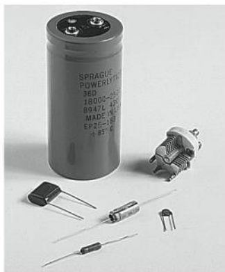
FIGURE 23.5 Typical capacitors. The large unit is an 18-mF electrolytic capacitor. At top right is an air-insulated variable capacitor in which one set of plates rotates to change the capacitance. The smaller capacitors range from 43 pF to 10 \mu F.
