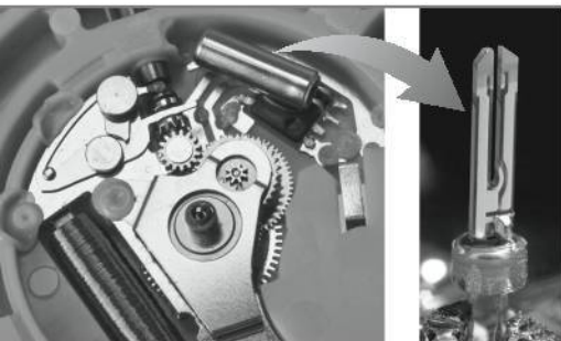
A tiny quartz tuning fork sets the timekeeping of a quartz watch. It oscillates at 32,768 Hz. What does this mean, and why this number?
