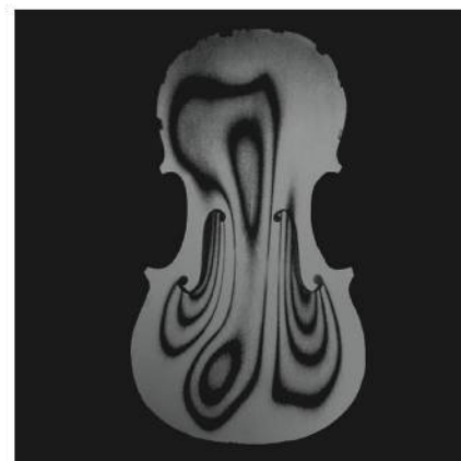
FIGURE 14.29 Standing waves on a violin, imaged using holographic interference of laser light waves.
