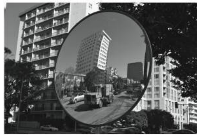
FIGURE 31.9 A convex mirror gives a wide-angle view.
