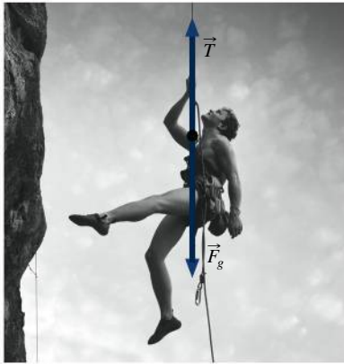
FIGURE 4.7 The climbing rope exerts an upward tension force \vec{T} that balances the force of gravity.
