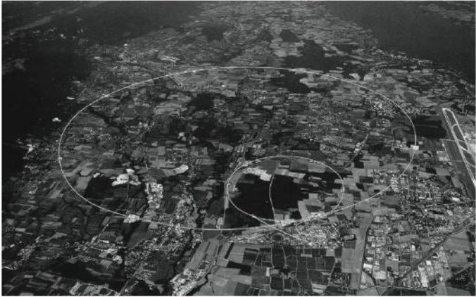
Aerial view showing the location of the 4.3-km-diameter Large Hadron Collider on the Swiss–French border. The accelerator itself is in a tunnel 50 m–175 m below ground. The device accelerates protons to 14 TeV. The smaller ring accelerates the protons to 450 GeV before they’re injected into the main accelerator.
