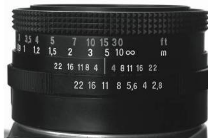
FIGURE 31.37 A 35-mm camera lens (Passage Problems 81–84). The numbers from 22 to 2.8 at the bottom are values for the f-ratio, f/d . Turning the ring with these numbers adjusts the iris that covers the outer part of the lens, thus changing the f-ratio.
