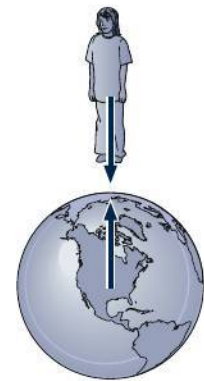
FIGURE 4.18 Gravitational forces on you and on Earth form a third-law pair. Figure is obviously not to scale!
